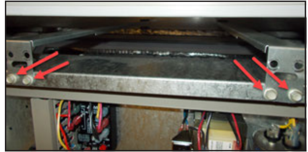
FIGURE 63 Remove Four Screws
