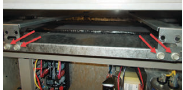
FIGURE 6 Remove Four Screws
