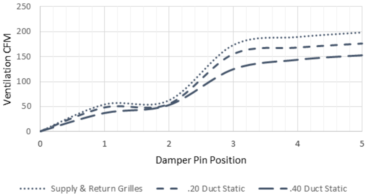
GRAPH 2 W24HF FAD-NE2, 3 W/O Exhaust Ventilation Delivery
