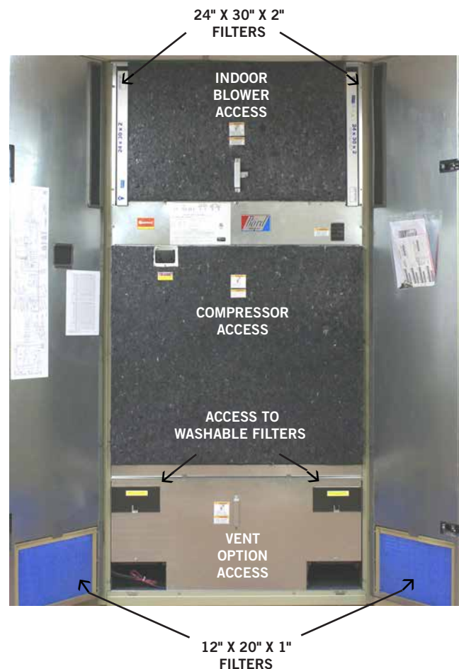
FIGURE 9 Filter Location
