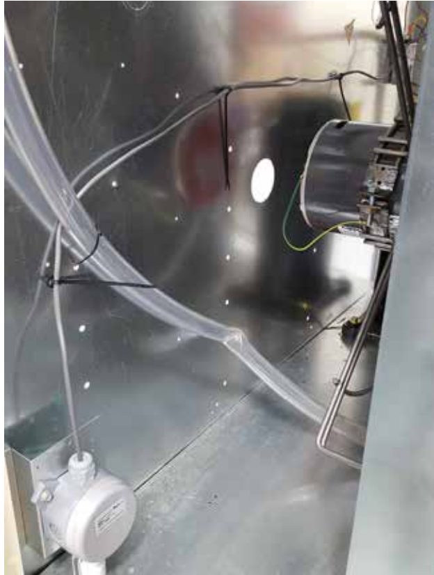
FIGURE 10 Wire Harness Secured to Back of Unit
