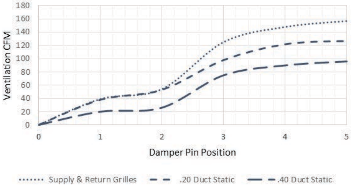
GRAPH 1 W18HB FAD-NE2, 3 W/O Exhaust Ventilation Delivery
