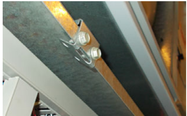
FIGURE 8 Re-Install Screws and Bend Tabs Up
