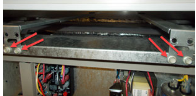
FIGURE 6 Remove Four Screws
