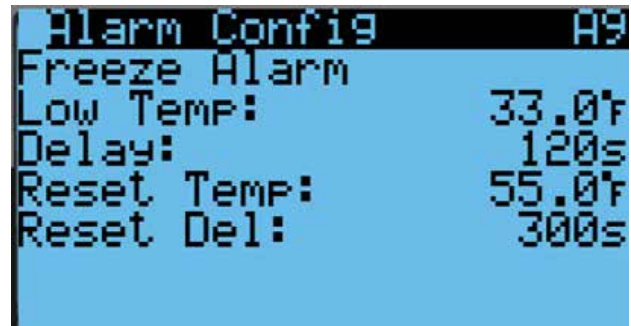
FIGURE 16 Adjusting Freeze Alarm Values
