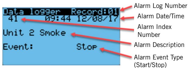
FIGURE 9 Alarm Log Screen Breakdown
