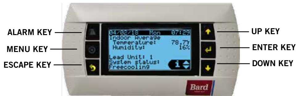
FIGURE 1 LV1000 Controller Display and Interface (Status Screen Shown)
