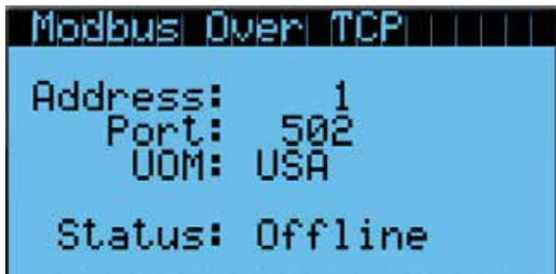
FIGURE 15 Modbus TCP Setup
