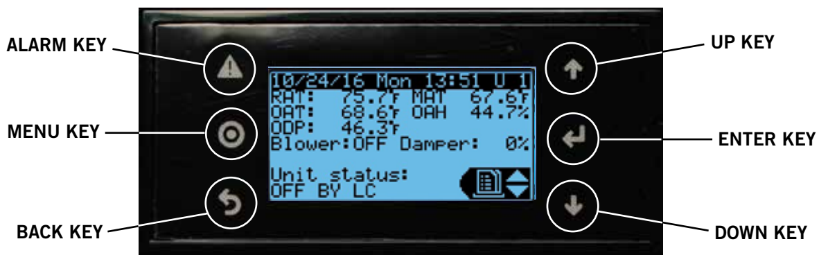
FIGURE 1.15 TEC-EYE™ (Bard P/N 8301-059) Display and Interface (Status Screen Shown)
