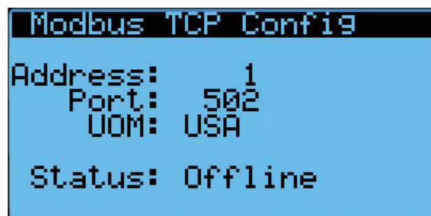
FIGURE 19 Modbus TCP Setup
